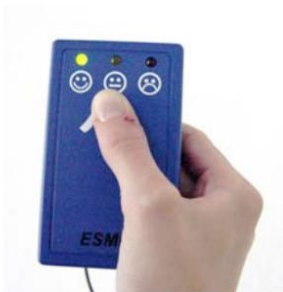
ESMINI Electrostress measuring device with traffic light principle
