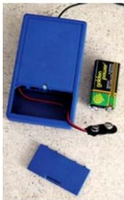
POWER SUPPLY WITH A COMMERCIAL 9V BATTERY
